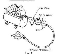
Use a 1/2" air hose between the compressor and the tool. Compressed air is cooled and its water content separated, as soon as the air leaves the compressor. A portion of the water content, however, is condensed in the-piping, and can enter the tool mechanism, and may cause trouble. So, install an air filter and an oiler between the compressor and the tool.
