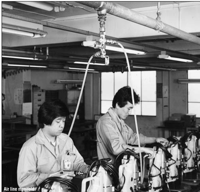
Air line manifold
