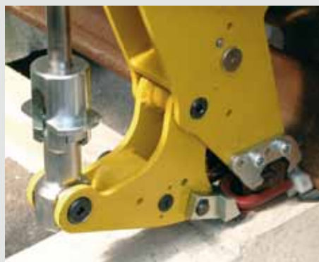
Extraction and insertion of Pandrol "Fast clips".
